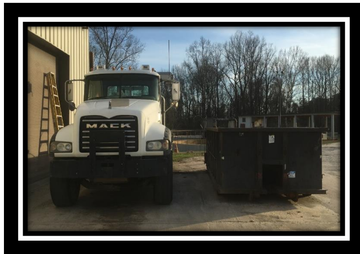
Sludge truck that is used to haul sludge to Lee County Landfill in a 30yard container
